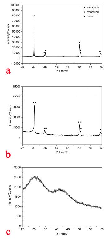
**Figure 4.** XRD images of zirconia surface from different groups: (a) For NT (no treatment group), the zirconia surface for NT was completely tetragonal-phase; (b) for APA (airborne particle abrasion group), the tetragonal phase ratio of the surface was low, with a small amount of monoclinic and cubic phases; and (c) for FSL (femtosecond laser group), there may be an amorphous phase, as it was also possible to form salt crystals on zirconia surfaces treated with FSL.
