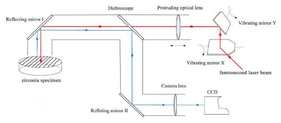
**Figure 1.** Schematic of the FSL surface treatment system and laser trajectory during surface treatment of the specimen. The red line indicates the propagation path of the FSL in the system, and the blue line indicates the light from the surface treatment result received by the charge-coupled device, which monitored the real-time processing results as the laser processed the specimen surface.
