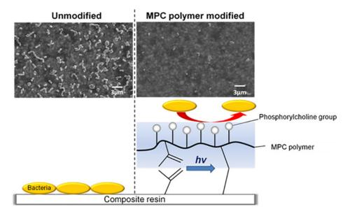
**Figure 4.** Schematic illustration of the use of 2-methacryloyloxyethyl phosphorylcholine (MPC) in resin composites. Adapted, with permission, from [93].
