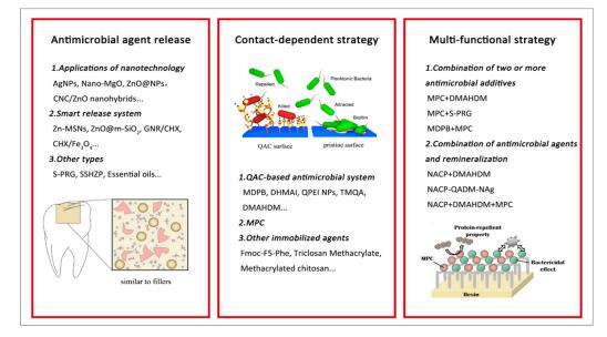
**Figure 1.** Examples of strategies for material composition modifications toward the design of antibiofilm resin-based composites. AgNPs: silver nanoparticles; MgO: magnesium oxide; CNC/ZnO: cellulose nanocrystal/zinc oxide; Zn-MSNs:
