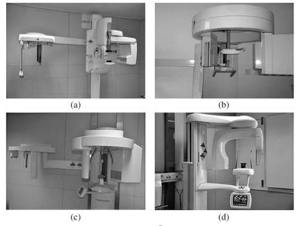
Figure 1 Images of the four panoramic machines (a) Orthopantomograph<sup>®</sup> OP200 (Instrumentarium Dental, Tuusula, Finland), (b) Orthophos CD (Sirona Dental Systems GmbH, Bensheim, Germany), (c) Orthophos XG Plus (Sirona Dental Systems GmbH) and (d) ProMax<sup>®</sup> (Planmeca Oy, Helsinki, Finland)
