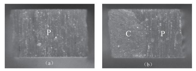
Fig. 3 Representative micrographs of the failure modes evaluation under the stereomicroscope at 80× magnification (C: cement, P: fiber post). (a). Adhesive failure displayed solely the impression of the fiber post surface over failure area. (b) Mixed failure displayed both the impression of the post and residual resin cement.
