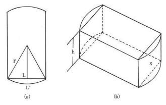
Fig. 2 Schematic illustration of the fiber post in the center of the microtensile test specimen. (a) The cross section of the fiber post in the center of the specimen (r=radius of the fiber post, L=chord length, L'=arc length). (b) The stereogram of fiber post in the center of the specimen. (h=thickness of the specimen, S=square measure of adhesion area). The square measure of adhesion area can be calculated according to the following formulas. L'=2r\*arcsin(L/2r), S=L'\*h
