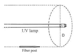
Fig. 4 Schematic illustration of UV irradiation. The UV irradiation energy on the post surface can be calculated according to the following formulas. I=w/[ $2\pi$ \*(r+D)\*L], E=I\*t. (I=irradiation intensity on post surface, E=UV irradiation energy on post surface, w=lamp power, r=radius of the UV lamp, D=distance between lamp and fiber post, L=length of the UV lamp, t=irradiation period).
